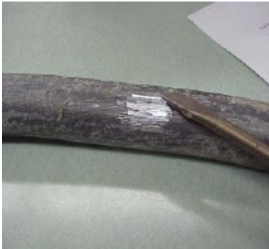
LEAD – Soft, will be shiny when scratched. Magnet will NOT stick to it.
