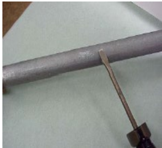
Galvanized Iron – dull steel color; magnet will stick to it.
